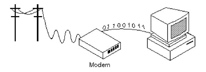
A modem is a device or program that enables a computer to transmit data over, for example, telephone or cable lines. Computer information is stored digitally, whereas information transmitted over telephone lines is transmitted in the form of analog waves. A modem converts between these two forms.
