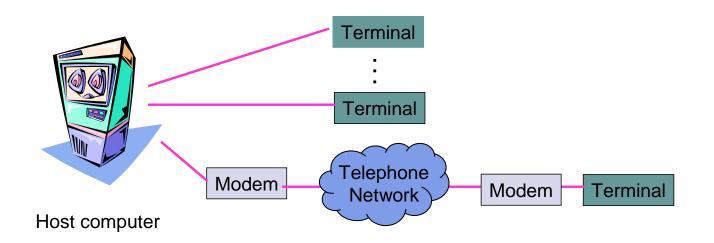
(\*) modem – device for sending digital data over phone line / analog network
