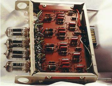
"Four dual triodes are used to count and store the 4 bits needed to represent a decimal digit. "
